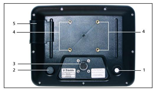
Figure 2.3 The back of the AgGPS FieldManager display unit
