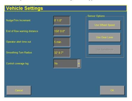
3. Enter a value in the *Nudge/Trim Increment* window. Use this increment to set the amount by which the **Nudge** buttons move the line back to the correct path, or by which the **Trim** buttons move the vehicle position.
