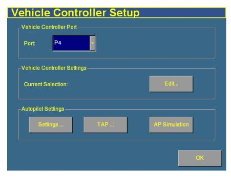
3. In the Port list, select the port on the FieldManager harness that the Autopilot controller is connected to.
