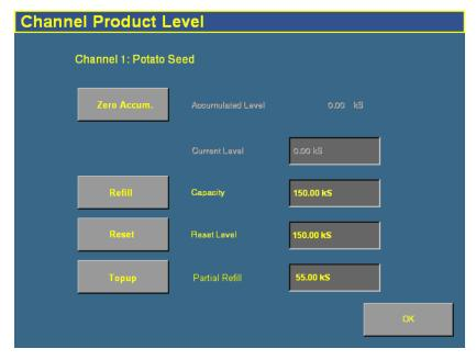
On this screen, you set the *Capacity, Reset Level*, and *Partial Refill* values, so you can quickly adjust the planter volume in the field.
