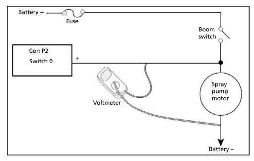
Figure 20.1 External boom switch connection
