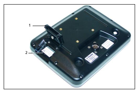
Figure 3.4 The reverse of the display with the card socket open
