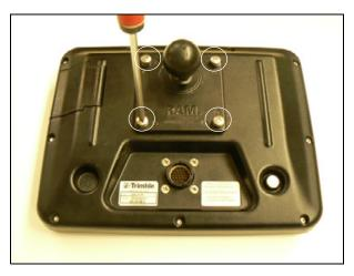
2. Attach the RAM mount to the ball on the mounting plate.
