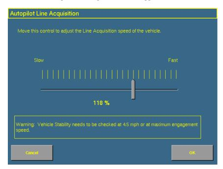
Adjust the line acquisition aggressiveness slider. The slider controls how aggressively the implement approaches the guidance line, using a scale from 50% to 150%. The optimal value for each profile is not necessarily 100%: it varies for different implement profiles.
