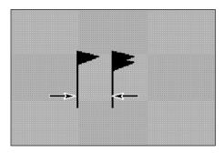
Figure 11.2 Right offset: Measure the distance between the flags
