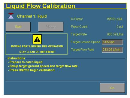
The *Liquid Flow Calibration* screen appears:
