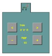
The TrueTracker tab enables you to adjust the implement steering independently of the vehicle steering. For example, if you can see that the implement is consistently to one side of the guidance line but the vehicle is correctly online, you can apply Trim to the implement to correct it.
