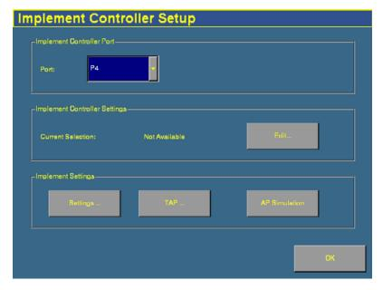
4. In the *Port* list, select the connector on the FieldManager harness that the TrueTracker implement controller is connected to.
