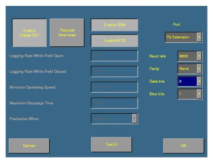
3. In the port list, select the port on the FieldManager display harness that the Enalta sensors are connected to.
