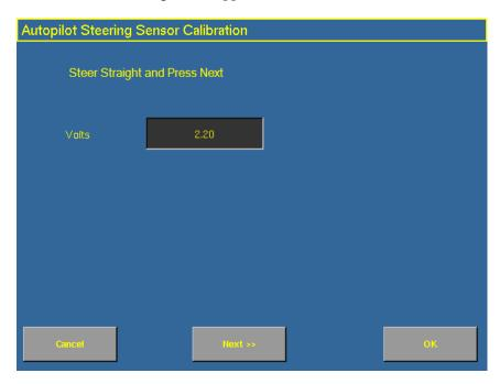
6. Center the steering wheel. While the wheel is at the center position, tap **Next**.
