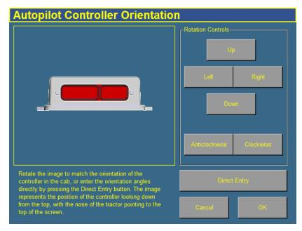
An image represents the current mounting orientation of the controller.
