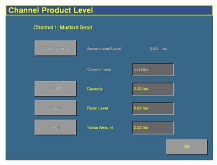
On this screen, you set the *Capacity, Reset Level*, and *Partial Refill* values, so you can quickly adjust the drill/seeder volume in the field.
