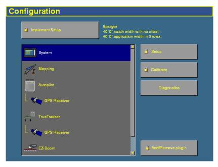
The currently installed plugins appear in the plugins list on the left of the screen.
