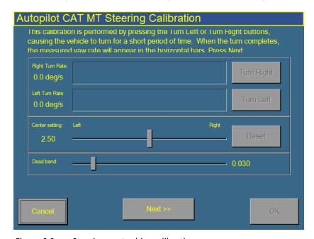
Figure 9.9 Steering center bias calibration screen
