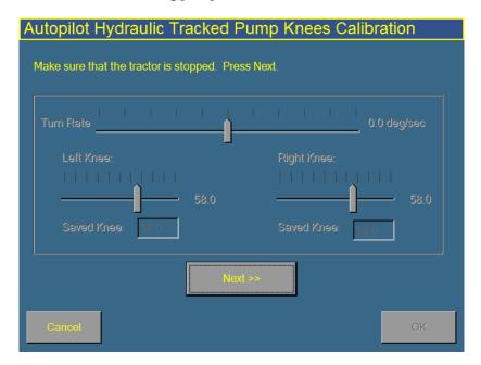
Figure 9.7 Pump Knee calibration screen
