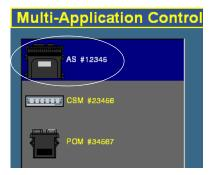
4. Ensure that the modules are shown in the list in the order that they are connected to the harness. The master module is not necessarily the first module.
