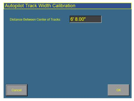
Figure 9.4 Track Spacing calibration screen
