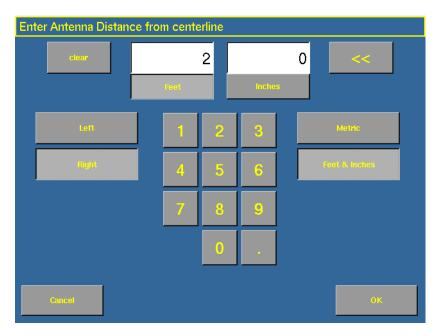
3. Enter this value into the *Antenna Distance from centerline* field and indicate whether it is left or right of the centerline. Values to the left of the centerline are displayed as negative numbers. The nose of the vehicle is considered the forward direction.
