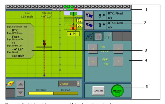
Figure 11.3 Main guidance screen with implement steering features
