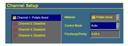
**Note** – The material being controlled must reflect the sequence of what is connected to the 4 channel control harness.
