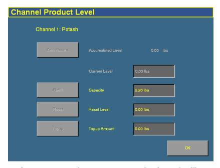
On this screen, you set the *Capacity, Reset Level*, and *Partial Refill* values, so you can quickly adjust the fertilizer weight in the field.
