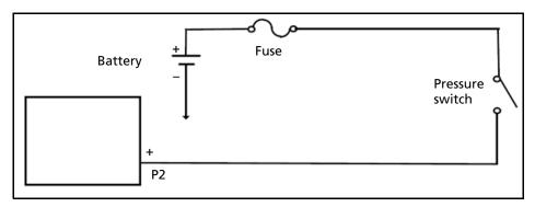
Figure 20.2 External pressure switch connections
