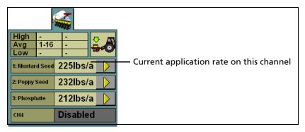
Figure 14.4 The air seeder product (channel) tab
