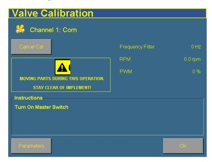
If you did not use the Limit Output function, turn on the Master switch. The calibration begins.
