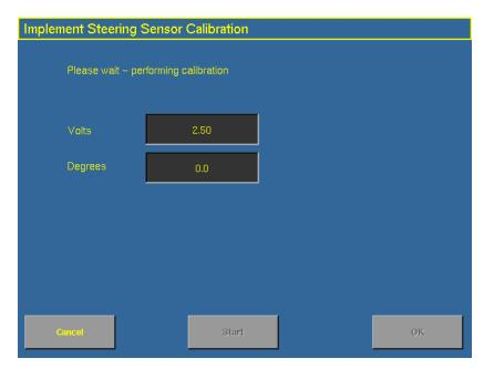
3. Perform the calibration. The value in the *Volts* field is updated as the wheels are steered.
