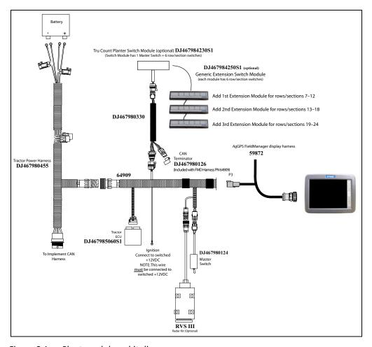
Figure 3.1 Planter cab base kit diagram
