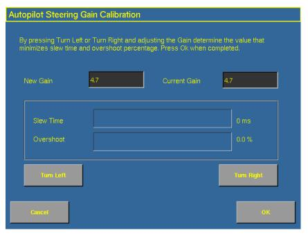
*Note* – *The optimum gain setting has short slew time (short millisecond reading) and low overshoot percentage (less than 5–8%).*
