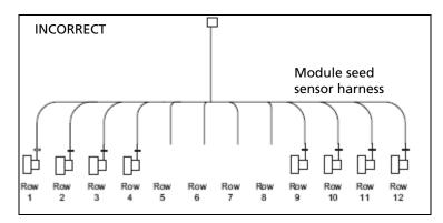
Failure to correctly install seed sensors will result in incorrect row assignment on the planter monitor display functions.
