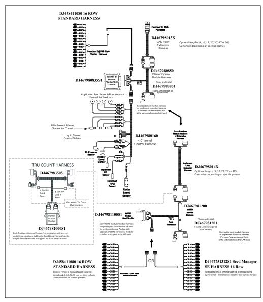
Figure 3.3 Planter monitoring and control system diagram: Implement CAN harnessing
