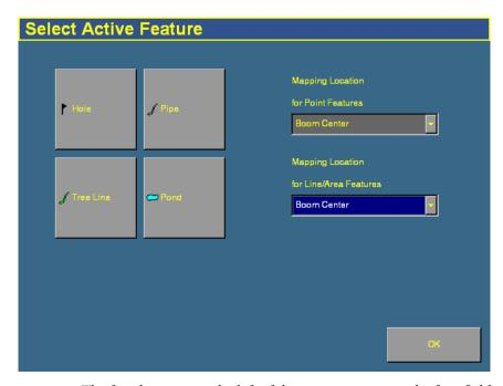
The four buttons on the left of the screen represent the four field feature buttons that appear on the *Mapping* tab on the Run screen (see previous page).
