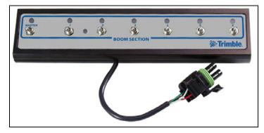
You can connect up to 4 switch boxes together so you have up to 24 switches. Install the switch boxes in a convenient place in the cab where you can comfortably reach them.
