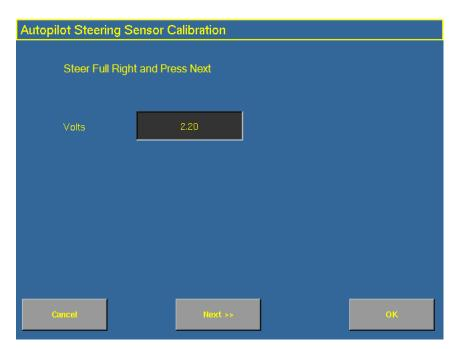
5. Turn the steering wheel completely to the right and then tap **Next**. If the steering wheel is not turned to the full right position or if the steering sensor requires adjustment or replacement, an error message appears.
