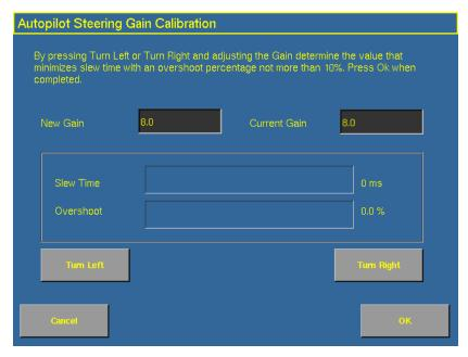
*Note* – *The optimum gain setting has short slew time (short millisecond reading) and overshoot percentage less than 10%.*
