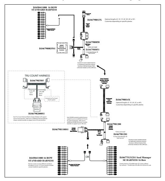
Figure 3.2 Planter monitoring only system diagram: Implement CAN harnessing
