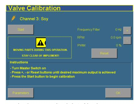
b. Press + or - to adjust the limit of the valve.
