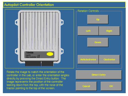
An image represents the current mounting orientation of the controller.
