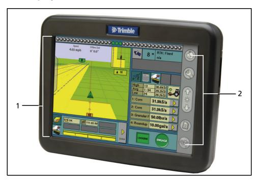
Figure 2.2 The front of the AgGPS FieldManager display unit
