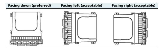
*Note – Do not install the module in any other orientation. The connection wires must not point upwards or dust and rain may enter the module.*
