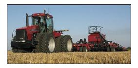
When controlled with the Multi-Application Control plugin, the air seeder can support up to 4 channels of material at once, enabling you to plant combinations of seed or to plant the seeds with liquid, granular fertilizer, or anhydrous ammonia.
