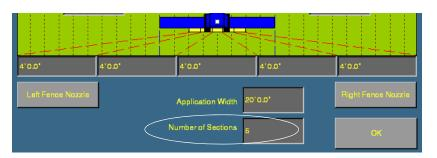
**Note** – The EZ-Boom controller supports up to 10 boom sections. If one fence section is enabled, you can have a maximum of 9 boom sections. If both fence sections are enabled, you can have a maximum of 8 sections.
