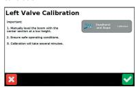
4. In the Deadband Calibration screen, tap to start the calibration process:
