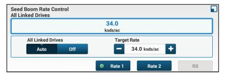
The "Rate Control" UDW is recommended on a Run Screen for adjusting rate while operating.
