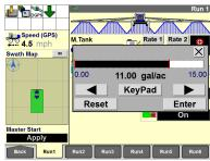
15 When using manual product control, press the target flow rate window. Press the arrow keys to adjust the pump speed.
