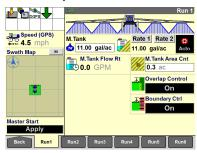
14 When using automatic product control, press the target application rate window. Press the bar graph or use the arrow keys to adjust the target rate.
